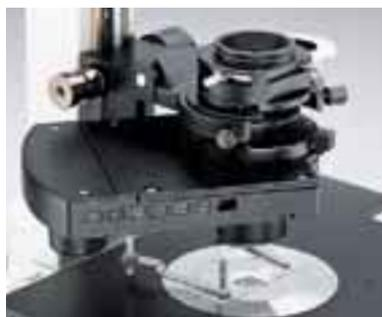
observations, while High Contrast (HC) prisms provide maximum contrast for thin specimens, and High Resolution (HR) prisms provide maximum detail with thicker specimens.
