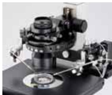
Unique Relief Contrast objectives feature rotatable modulators for constant shading for all magnifications.
